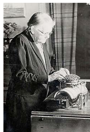
Left: A "writing ball typist". This writing ball from 1875 was rather high and should therefore be placed on a relatively low table in order to have a good typing position. Centre: Malling-Hansen's invention underwent continuous improvements, and can be found in a variety of versions. Presumably, old "balls" were disassembled and mounted on newer models. This is the model that was developed by mechanic August Lyngbye in 1885. Photo: Dieter Eberwein. Right: The publications for the writing ball claimed that it could be used by anybody, even persons suffering from trembling hands.
